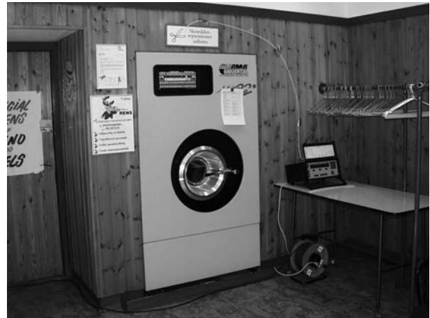
The front of the dry cleaner machine, the note list and the monitor for PCE.
